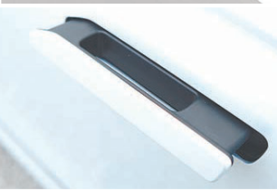
Retractable door handles improve aerodynamics.
