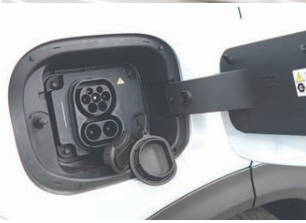
The J7 PHEV can be recharged with AC and DC charging.
