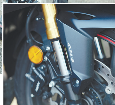
The front suspension is upgraded with 37mm Showa Separate Function Forks.
