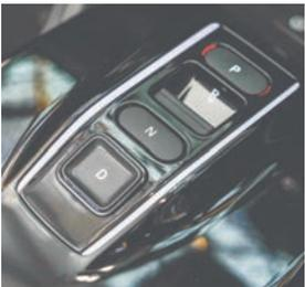
There’s no gear knob in the traditional sense, just gear selector buttons.
